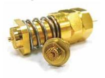
The integration of sense pin and force pin form into coaxial pin. Force pin is designed in one piece to endure higher current.
