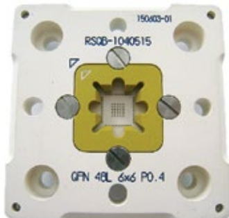
QFN Socket Pitch 0.3mm
