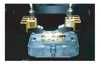
CCP has a dedicate high frequency lab that uses TDR, network analyzers and RF probe stations to measure the socket / pins actual performance and therby verifying the simulation results.
