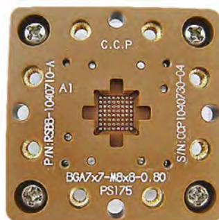
BGA Socket Pitch 0.8mm
