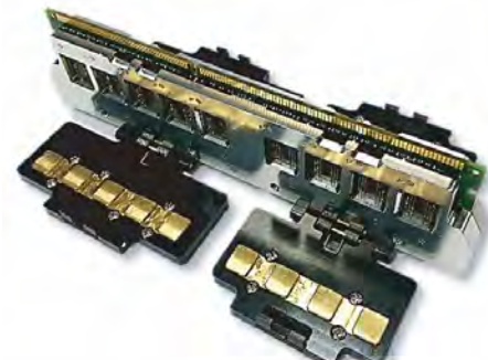
Manual DDR3 Testing Module Double Side
