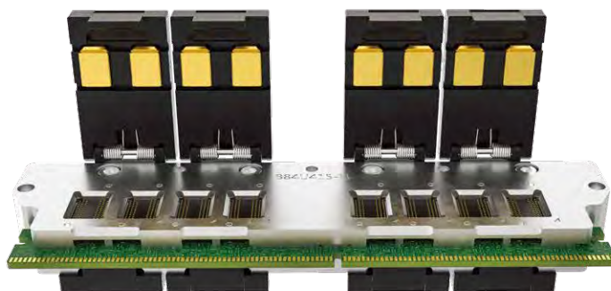
Manual DDR2/3 Testing Module Single Side
