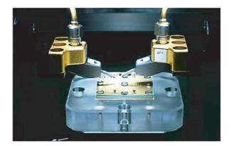
CCP has a dedicate high frequency lab that uses TDR, network analyzers and RF probe stations to measure the socket / pins actual performance and therby verifying the simulation results. These are all indispensable equipments for developing new high-class products.
