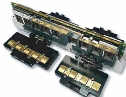
Manual DDR3 Testing Module
