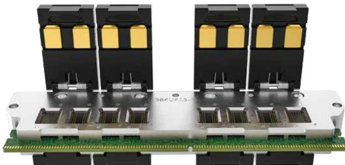
Manual DDR2/3 Testing Module
