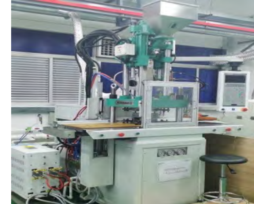
55T-120T Injection Molding Machine Capacity: 3KK pcs / Month
