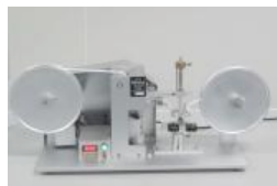
RCA Tape Abrasion Tester
