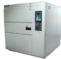
Thermal shock test machine
