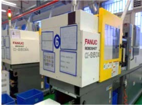
50T FANUC ROBOSHOT Injection Molding Machine Capacity: 3KK pcs / Month
