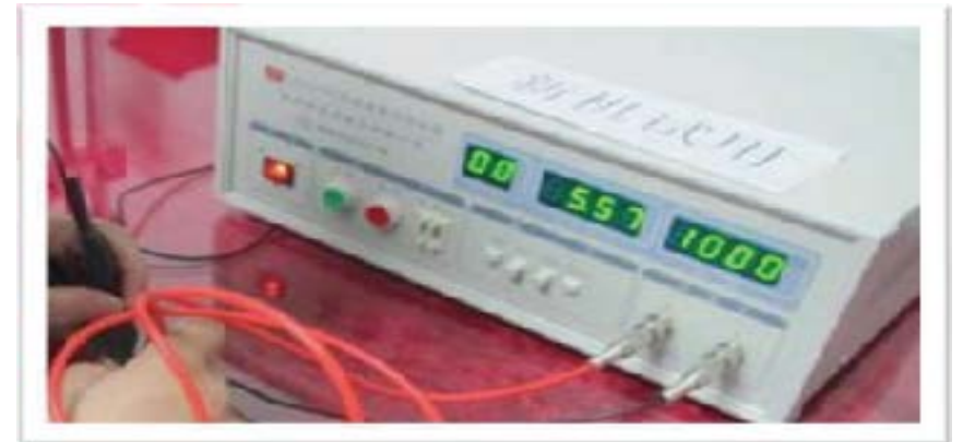
Insulation Resistance Test (LK2679D)
