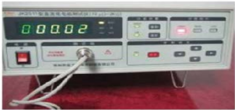
DC Resistance Tester JK2511 (10 \mu\Omega —2K \Omega )
