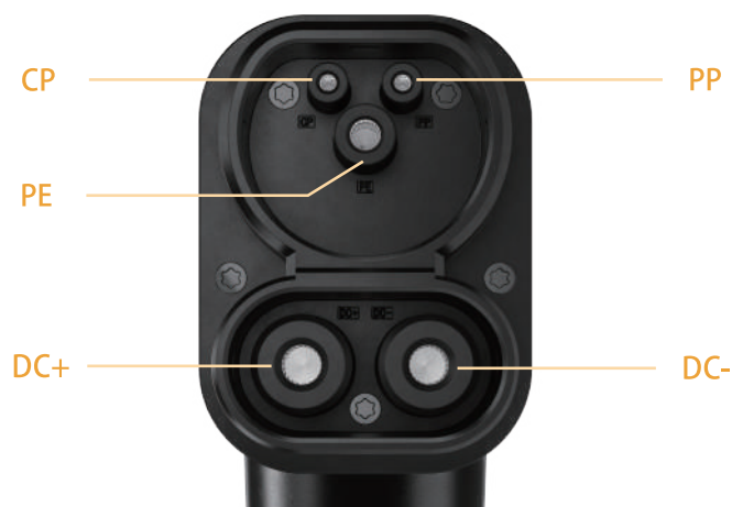
CCS2 IEC 62196 DC Vehicle Connector
