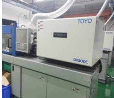
50T-170T TOYO DH300C Injection Molding Machine Capacity: 5KK pcs / Month
