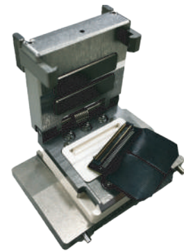
Dual-site pogo socket with fine pitch connector (DUT)
