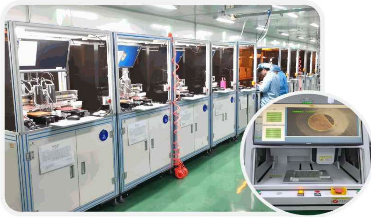
Pencil B222 auto assembly line with cosmetic inspection AOI
